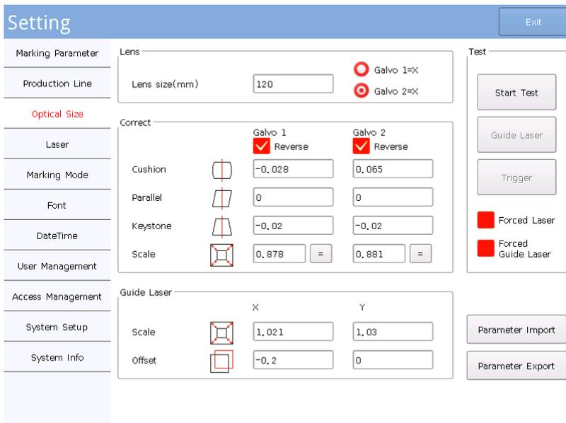
Area size: the size of the work area size, the general set to the lens corresponding to the actual maximum marking range
