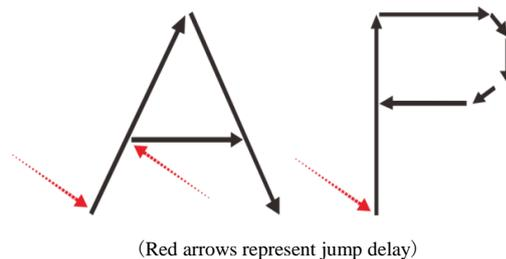
**Corner Delay:** Definition: (Unit:  $\mu s$ ). Refer to the time delay of mirror signal at the character corner. (Range of 30-200).
