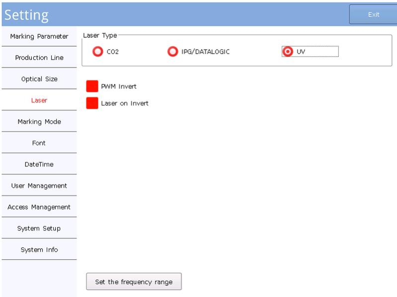
When the device is equipped with UV lasers should choose the type of UV lasers.
