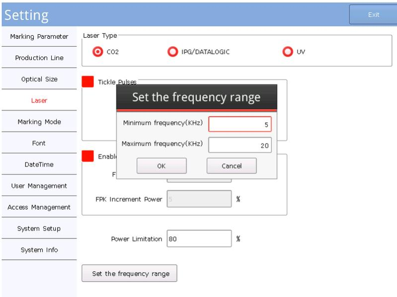
**Frequency range setting:** When using this type of laser, it is used to set the minimum and maximum frequency of the input in the parameter.
