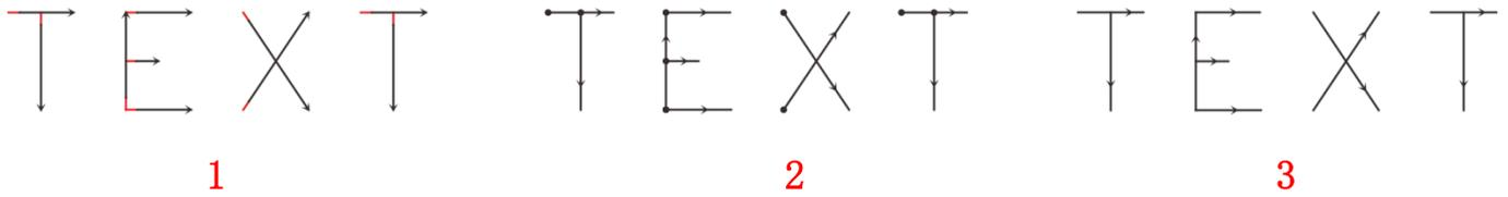
Case 1: There is no laser on the line section of beginning end (red line is the line section without laser) as shown in the figure below. It's caused by too long laser on delay, so the laser on delay shall be shortened;
