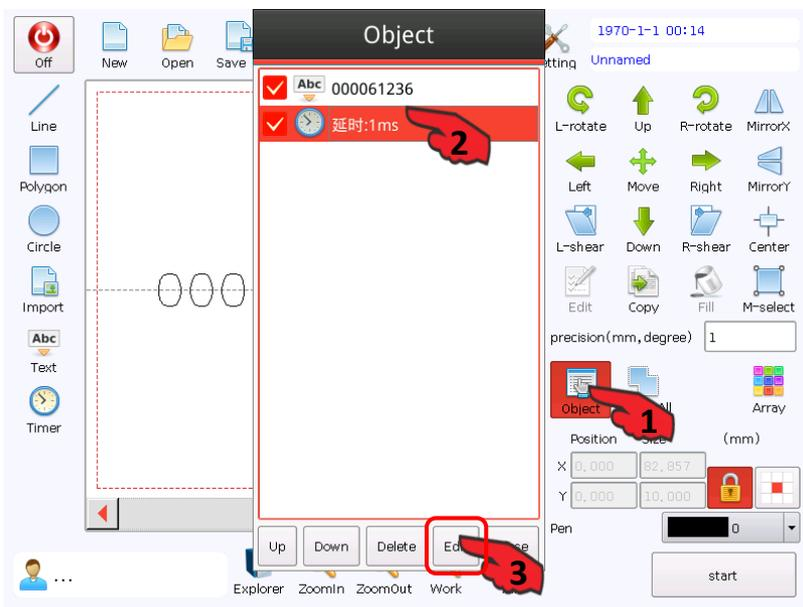
To change the delayer, select the delayer to be changed from the “Object List”, and then click “Edit” at the bottom of the “Object List” and then change the delay value in the window popped out.
