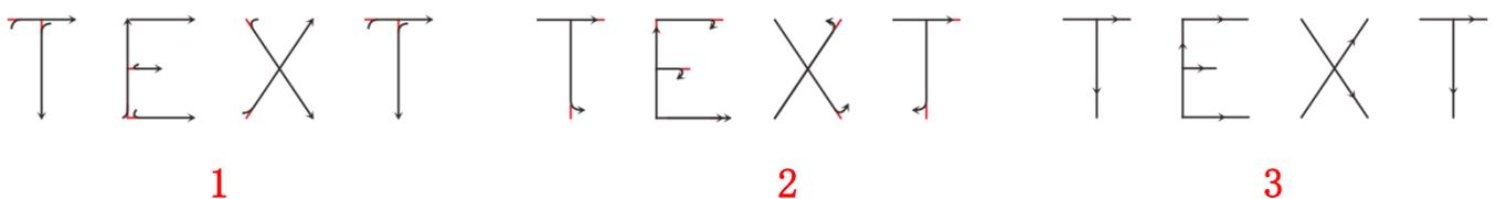
Case 1: The beginning line is deformed, at this time; the jump delay shall be prolonged.
