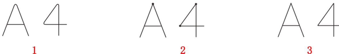
Case 1: As shown in the figure above, the graph with sharp angle required turns to arc angle. It’s caused by too short corner delay, so the corner delay shall be prolonged.
