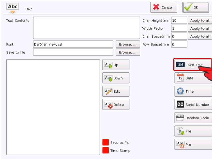
**Save to File:** Tick it to save the marking content in a .txt file.
