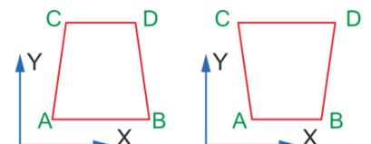
And then measure the length of the two vertical lines, that is, the AC line and the BD line. If the length of the AC line is smaller than the length of the BD line in the first case, the coefficient of the corresponding Y-axis of the Y axis is smaller. In both cases, the coefficient of the corresponding Y-axis of the Y-axis is changed.
