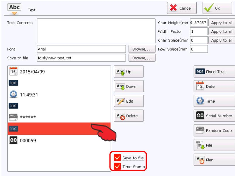
Select the “fixed text” (New Line) between the random code and serial number, tick “Save to file”, and then the file name and the file path are consistent with the random code and serial number.
