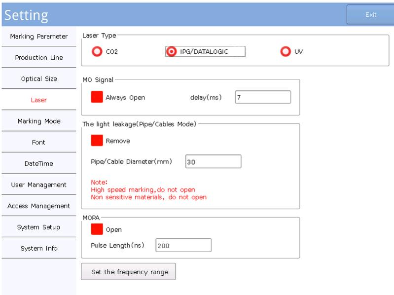
When the IPG / DATALOGIC laser type is selected, the setting window on the left side appears. This laser type is compatible with Chong Xin, Ruike and joint products such as DB25 core interface type of laser.
