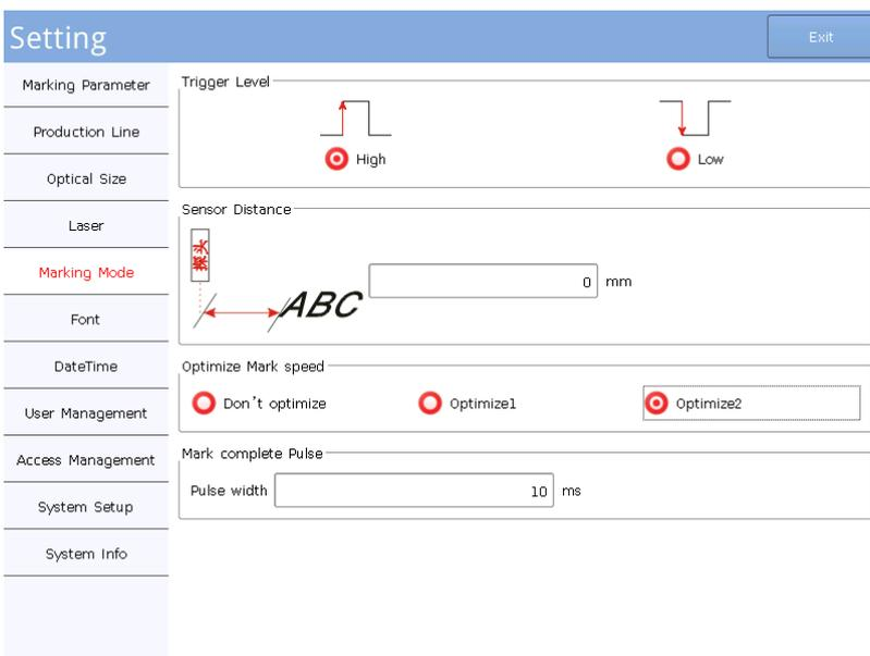
**Trigger Level:** Select high or low level of external trigger input, both of which are edge triggered (rising edge or falling edge trigger).
