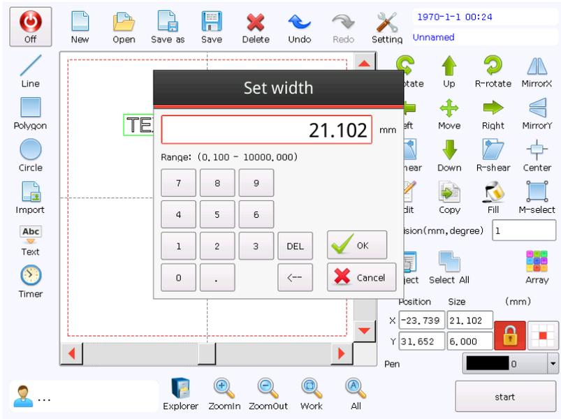
Click the size (X-width, Y-height) and input corresponding value in the dialogue popped out, and click “OK” to change the value. If the X-Y is locked, to change a value, the other value will be zoomed automatically. If the X-Y is unlocked, to change a value, the other value will not be changed.
