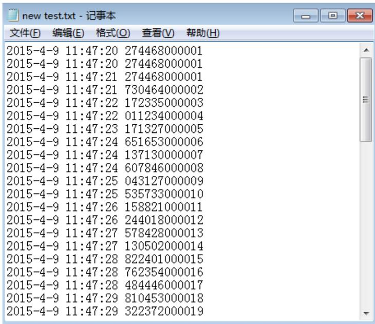
The left figure shows the rendering that the random code and serial number file is opened. As shown, there is no “blank space” between the random code and serial number. To separate the random code and serial number with a “blank space”, save the fixed text “newline” of the two in the marking file in the same file.
