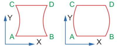
And then look at the two lines that AB line and CD line is a straight line, if the first case on the right, then the Y axis corresponding to the galvanometer coefficient smaller; if the second case, the Y-axis corresponding The coefficient of the galvanometer is changed.
