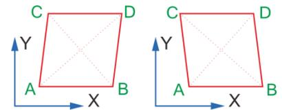
If the length of the AD line is less than the length of the BC line, the coefficient of the Y-axis corresponding to the galvanometer is changed. If the second case occurs, the coefficient of the corresponding Y-axis of the Y-axis is changed The.
