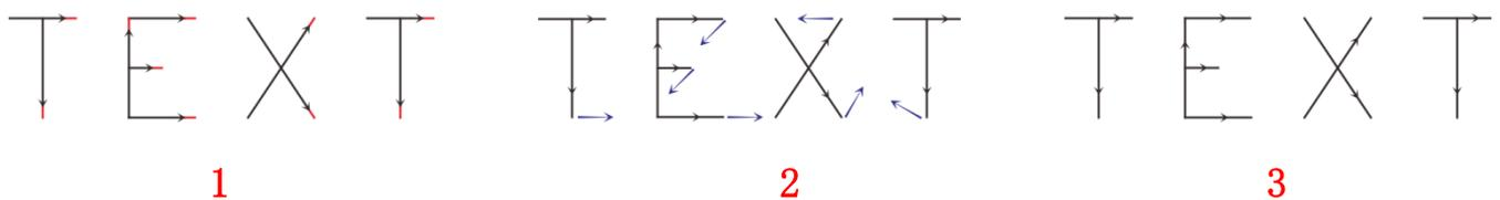
Case 1: There is no laser on the line section of end (red line is the line section without laser) as shown in the figure below. It's caused by too short laser off delay, so the laser off delay shall be prolonged;
