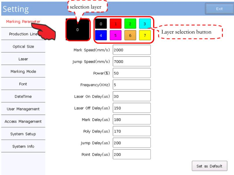
**Marking Parameter:** A color marks a parameter and different colors mark different marking parameters rather than the color of marking.
