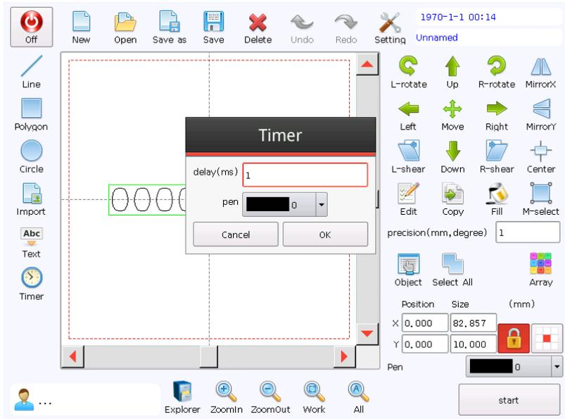
During marking, as required, add a delayer, with unit of “ms”, 1s=1,000ms=1,000,000us.
