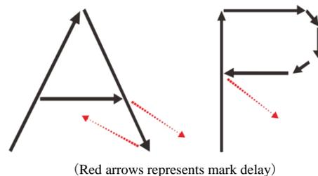
**Jump Delay:** Refer to the time delay for laser jumping between characters.
