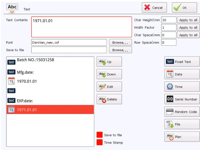
The left figure shows the rendering after the “Exp. date” is added, the date behind the “Exp. date” is 365 days (one year) later than the current date.
